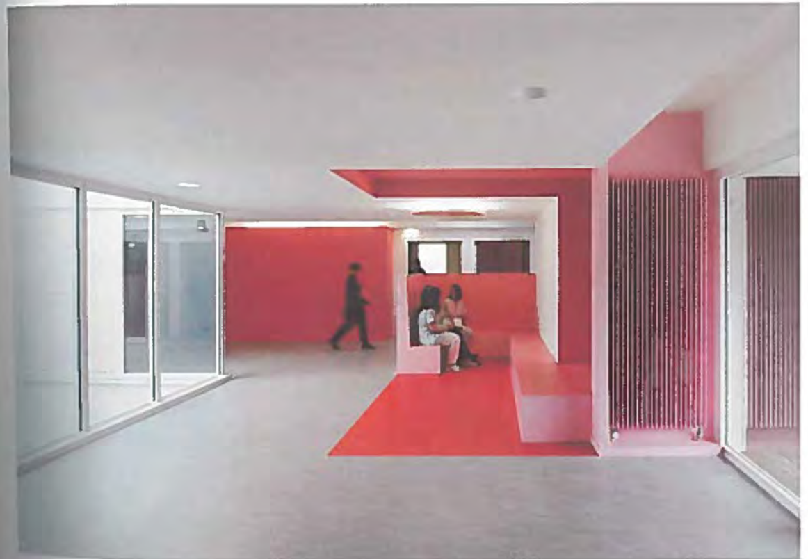
maat architettura, Apartment, Turin, Italy, 2006. Epoxy resin coating on floor and wall, satin finish, color code: SIKKENS G8.30.85 (4041 color concept)
